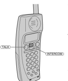
The base phone and cordless handset ring and "\*\* INTERCOM 1 \*\*" appears on the display of the base phone and "\*\* INTERCOM 0 \*\*" appears on the display of the cordless handset.
